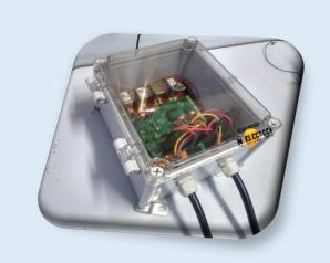
IOT based Controller Box - IP67 Mount
